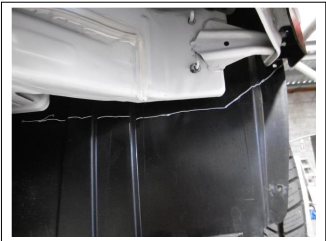
Figure 5: Trim line on left hand liner.
