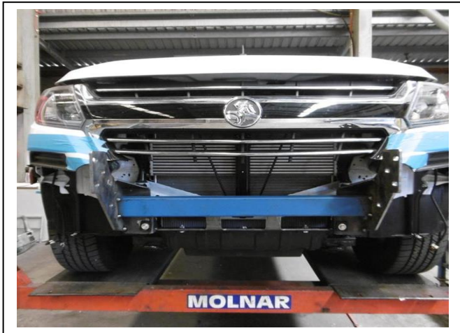
Figure 13: Cut across grille to fit over steel mount leaving grille mount on grille.
