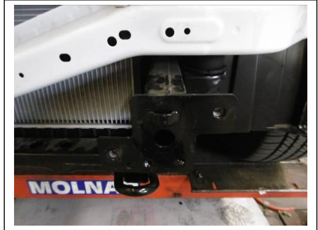
Figure 8: Flatten down tab.
