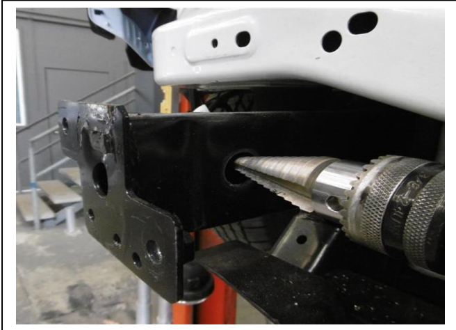
Figure 7: Enlarge hole to fit tube spacer.
