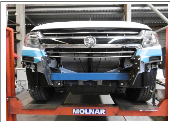
Figure 9: Steel mounting bracket fitted.
